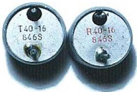
It is important to identify which is which as any subsequent results may suffer. The transducers used were clearly marked on the underside, but I am unsure if this is a common practice among these types of transducers.
