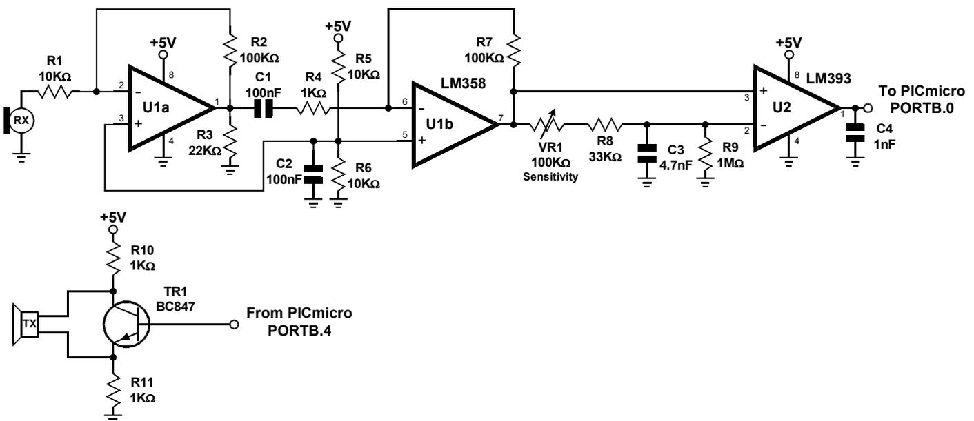
As you can see, the circuit is remarkably simple, consisting of two ICs (U1a and U1b are in the same 8-pin package) and a handful of common value discrete components.
